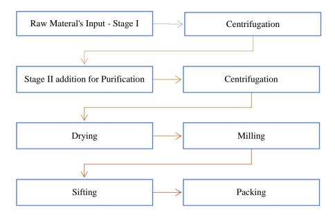
The process flow chart of other products manufactured by the Company, on demand basis, is given below. The quantity produced completely depends on the orders received.
